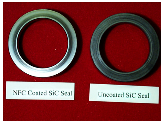
Figure 8. General view of NFC-coated (left) and uncoated SiC seal after 200 h tests.
